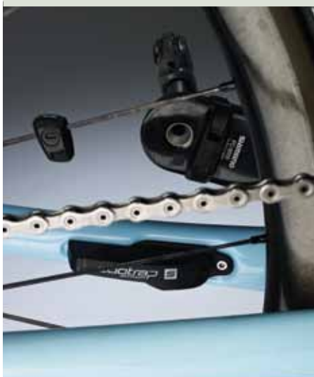
Trek’s new Duo Trap S is one of the neatest solutions we’ve seen for integrating data capture into the frame design. The sensor, sitting almost out of sight within the confines of the left chainstay, allows both a wheel magnet and crank magnet to calculate your speed and cadence. The latest version works on both ANT+ and Bluetooth platforms, which means it will pair with just about every device on the market. It’s further evidence, along with the Blender bar mount and the integration of the 3S chain catcher, that Trek is thinking about every aspect of the ride and minimising the clutter associated with current trends.
